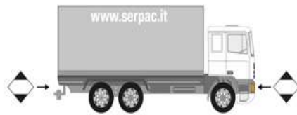
Limited Quantity (LQ) Vehicle Carrying over 8 Tons
